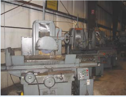
Gallmeyer & Livingston Grinders No. 560 14" x 36" No. 460 14" x 24 1/2" No. 376 12" x 24" K.O. Lee 6" x 18" Dry Grinder
