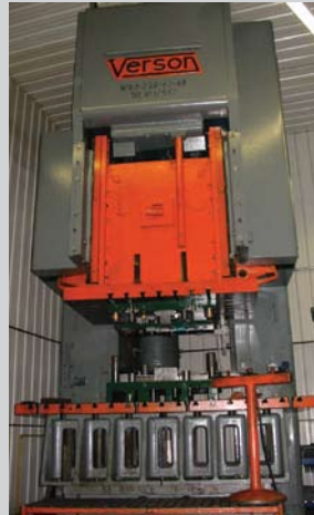
250 Ton Verson Gap Frame Press With 48" x 72" Bed Up to 48" Shut Height
